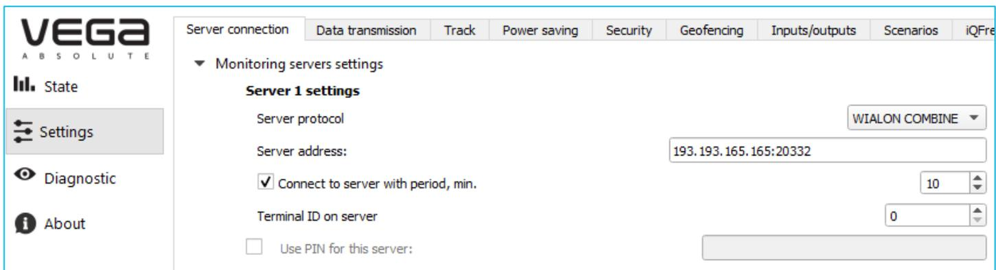
The screenshot shows the Vega Absolute settings interface. The 'Server connection' tab is active. Under 'Monitoring servers settings', 'Server 1 settings' are visible. The 'Server protocol' is set to 'WIALON COMBINE'. The 'Server address' is '193.193.165.165:20332'. The 'Connect to server with period, min.' checkbox is checked, with a value of '10'. The 'Terminal ID on server' is '0'. The 'Use PIN for this server' checkbox is unchecked.
