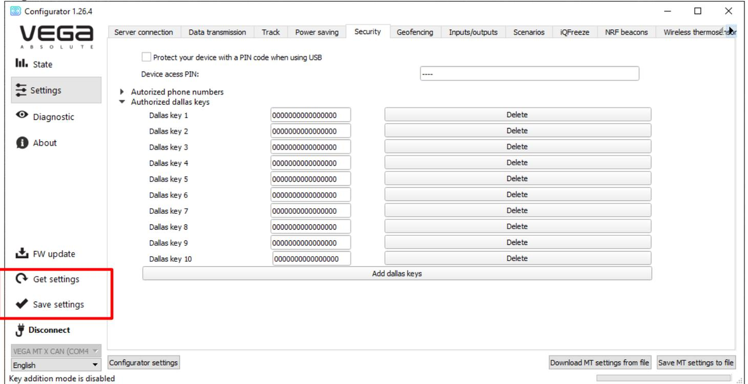
The “Configurator” program has the functions of saving settings to a file and loading settings from a file with the \*.vsf extension. The corresponding buttons are in the lower right corner of the program window. This function can be used both to speed up the process of setting up several devices of the same type, and when contacting technical support for a more informative description of occurs.
