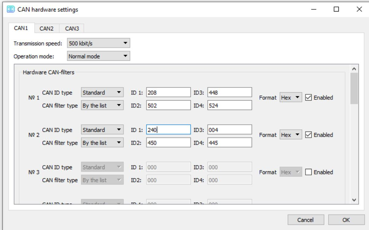
**Transmission speed** – it is important to indicate the correct speed for a CAN bus.
