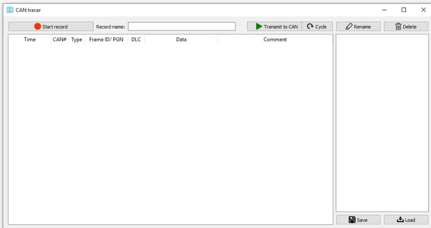
When you click on the "Start Record" button, all information coming from the CAN-bus in real time will be recorded in the stream mode and displayed in the window. In this case, the "New Entry" will appear in the field on the right - the name can be changed. After the recording is completed, you can write the
