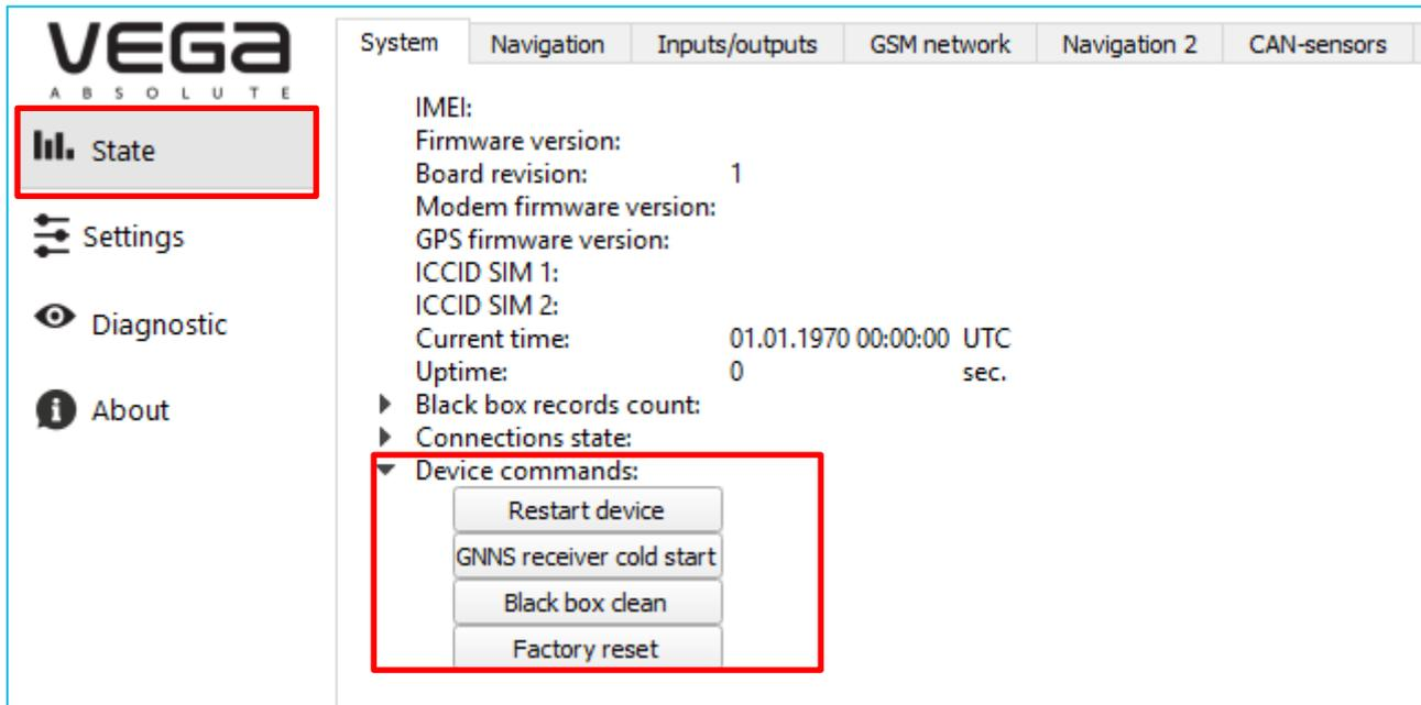
**Restart device** – forced device reload. In this case, the connection with the device will be lost and it will need to be reconnected to the "Configurator".
