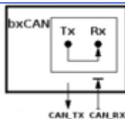
In this mode, all packets will be returned to the device without going to the CAN bus.
