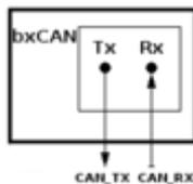
Data is transmitted and read from the CAN bus in normal mode on both sides.
