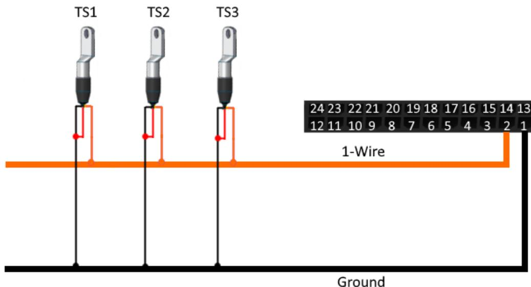
For the device to recognize the connection of a new sensor, it is necessary to connect to the device through the "Configurator" program (see "Settings" part), go to the "Inputs/outputs" tab and select the "Dallas temperature sensors" setting item.
