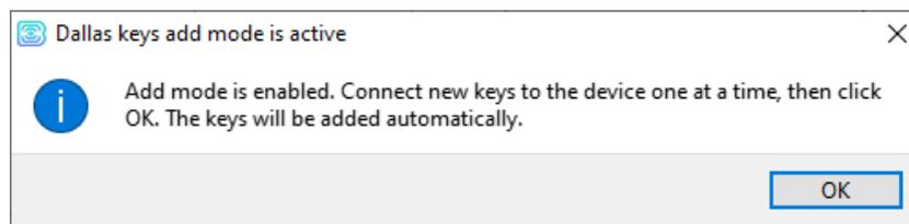
Attach the key to the reader as during authorization - the device will remember the key number - and click "OK". The key number appears in the free field. If several keys are added at the same time, it is allowed to attach them to the reader in turn, while the add window is open, and only then click "OK" - the numbers of all keys will be added to the free fields in the order in which they were applied to the reader.
