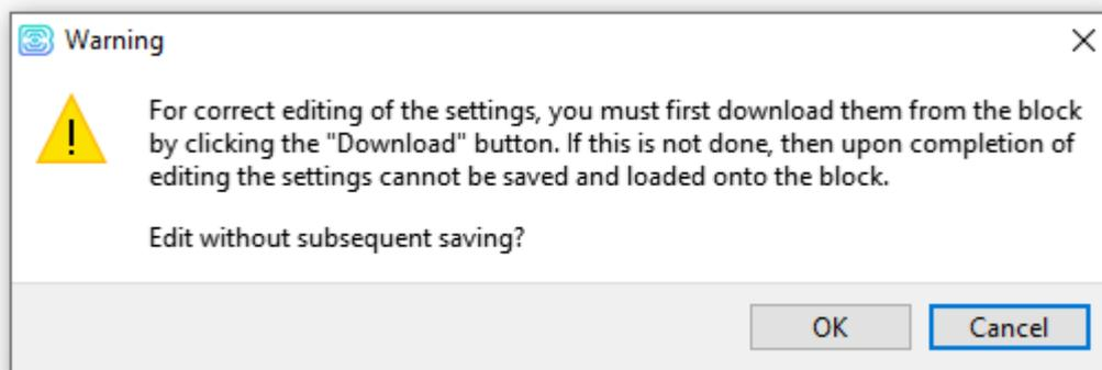
It also appears if the device was not connected at all. Therefore, before configuring CAN sensors, you need to load the settings from the device by clicking the "Download" button in the left part of the window.
