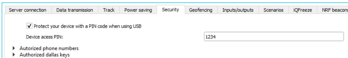
Protect your device with a PIN code when using USB – if there is a checkmark - when you start the "Configurator" program, when you try to connect to the device, you will be asked for the PIN code specified in the field on the right; if unchecked - when trying to connect to the device, the PIN code will not be requested.
